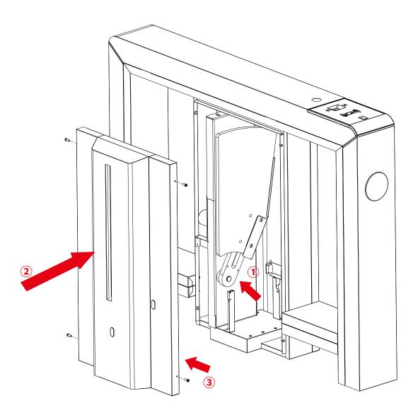
**Note:** The swing arm is already installed in the factory.
