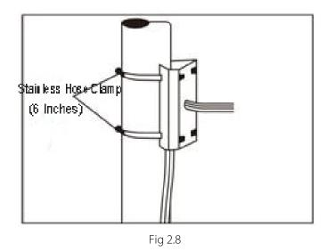
b. As shown in fig 2.9, fix the wall hanging bracket with all cables through it on the pole mounted attachment.
